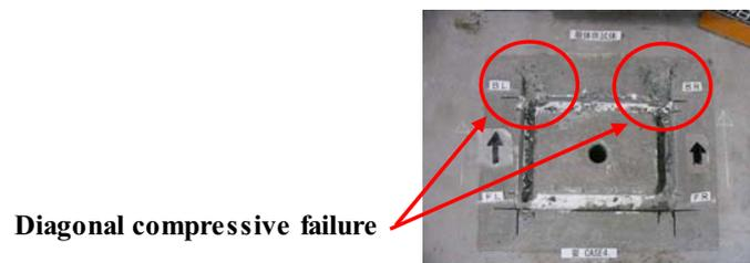
Photo.3 Failure modes of the specimen for the concrete structure
