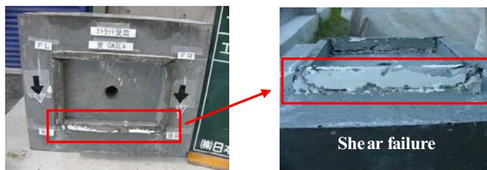
Photo.2 Failure modes of the PCa cradle
